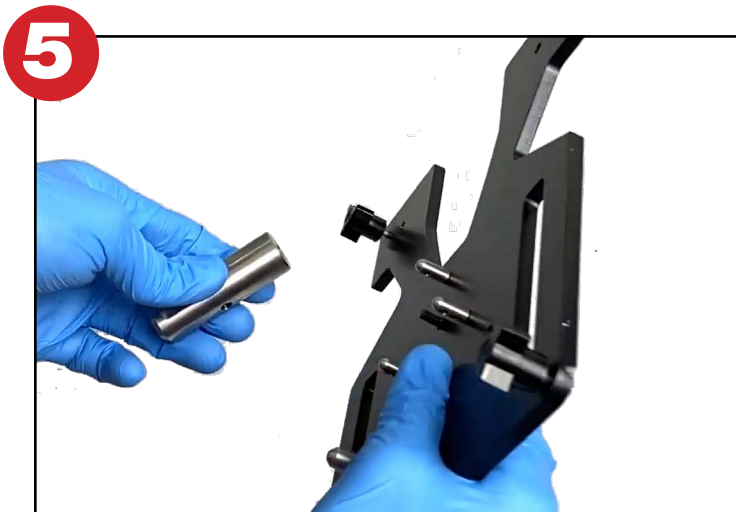
Step 5: Remove the pin from the assembly. Keep the allen key and screw.
