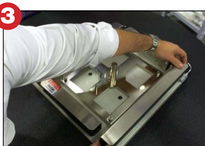
Step 3: Place the side 15" Gripper Channels just inside the Hoop Ring and down the side of the Adult Platen. Ensure the side Gripper Channels are installed approximately 1/4" from the edge of the platen.
