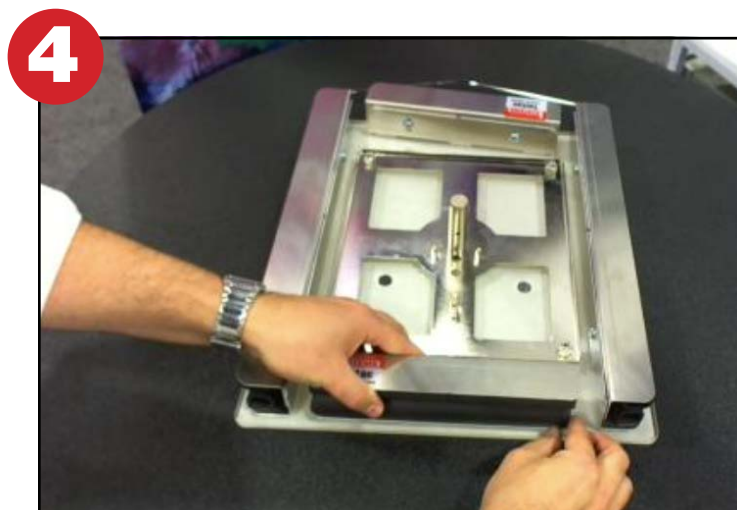
Step 4: Center the front and back 9" Gripper Channels between Side Gripper Channels. Ensure the front and back Gripper Channels are installed approximately 1/4" from the edge of the platen.
