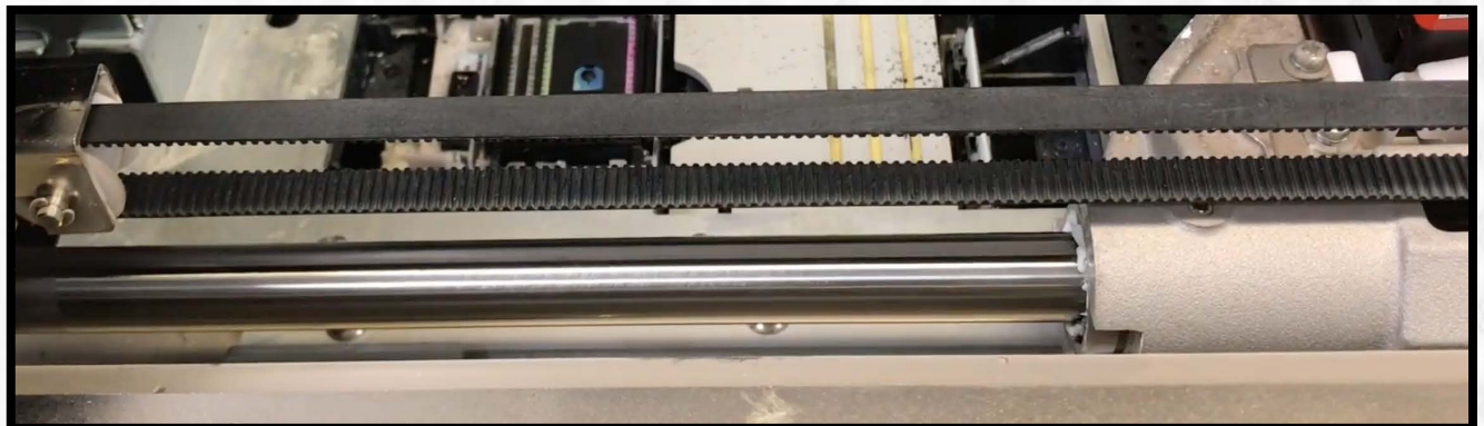
Print head carriage Encoder (Front) Rail
