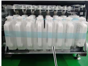
Cushioning material between tanks
