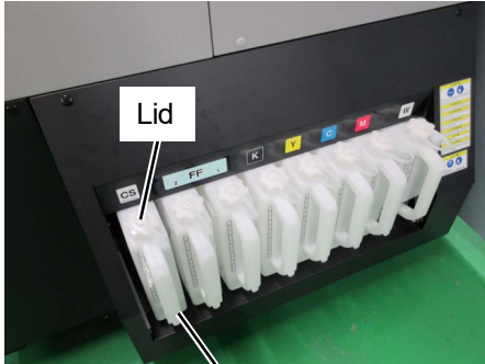
Cleaning solution tank
