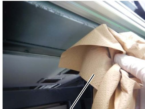
Wipe off the adhered mist ink with a waste cloth
