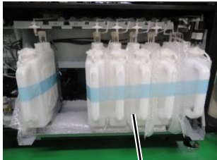
Cushioning material between tanks
