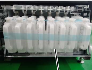
Cushioning material between tanks
