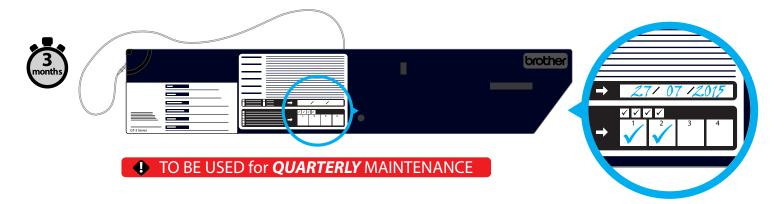
This **Maintenance Cartridge for CMYK** should be used to perform the **CTC** every **three months**. It is the only way **to clean** easily all the little **color tubes inside** the Maintenance station and keep a good suction of the pump to clean PrintHeads. > It is also a consumable like the MNT Cartridge for White. Mark the date or check the 5L bottles.
