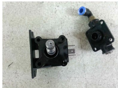
(P12-7) Disassemble to top and body
