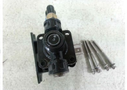
(P12-6) After removing screws
