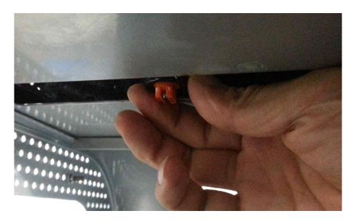
6. Either using a pair of pliers or by hand to adjust the nozzle until it is straight to assure an even spray area.
