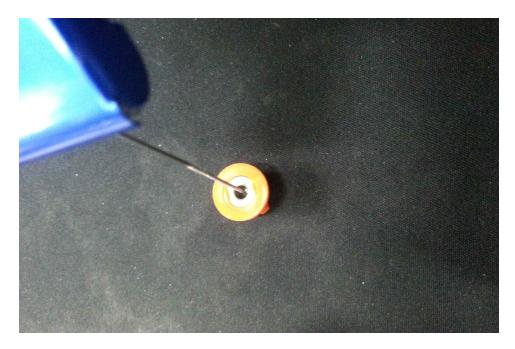
4. Using the cleaning brush provided with the machine brush the tip of the nozzle to help dislodge any debris and the rinse it under running water.
